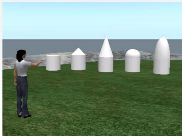
Locating each one on a scale shows the effectiveness of the various types of nose cone shape with regard to drag. On the left we have the % of flat face drag and not surprisingly the flat end nose cone has the highest value of 100% with a drag  $C_d$  of 1.5; notice that the drag coefficient is just a number it has no dimensions.
