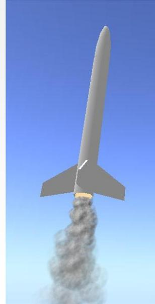
In this image the rocket is clearly veering away from a vertical path, but this is not necessarily caused through the influence of weather cocking to a side wind. Here it's possible that fins have been installed that are poorly aligned and positioned. An equally dramatic effect may arise from rough unsmoothed joints such as those between the fin and body causing airflow turbulence.
