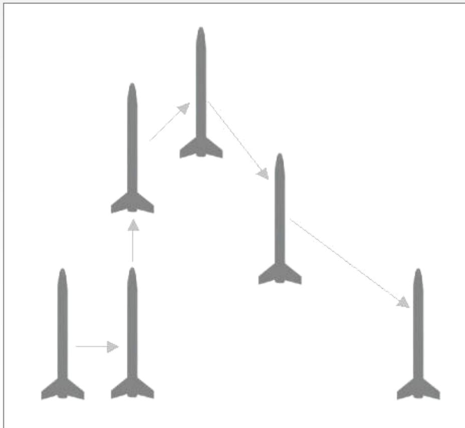
When considering how high a rocket or far a rocket can travel then we are referring to its translational motion, but considering stability then we must consider this in terms of rotational motion.
