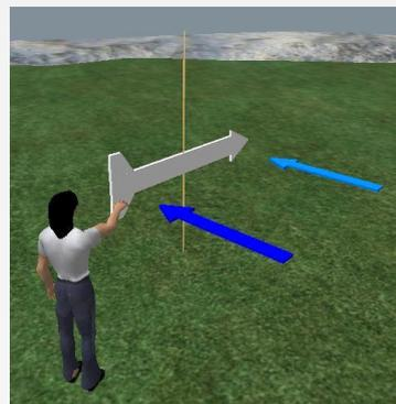
Here you can see how the unequal distribution of wind resistance at either end of the weathervane has caused it to face into the direction of the wind.
