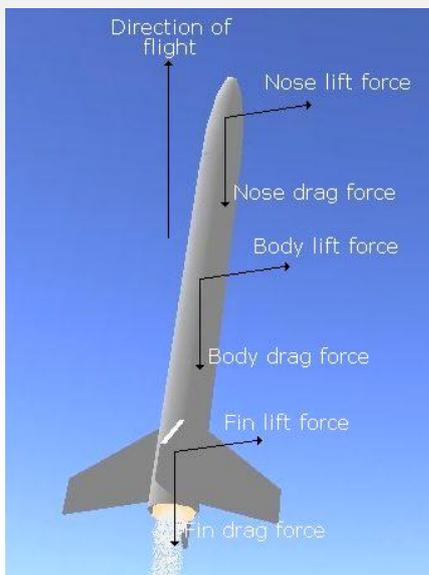
From our understanding of Static Stability we can now appreciate that during the course of a rockets flight all the major components; nose cone, body and fins are able to produce both lift and drag. The point of balance for all of these combined forces is the Center of Pressure
