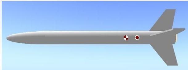
A final practical pre-flight assessment of your rockets stability is the swing test. Here you secure a tether to the main rocket body at the center of gravity mark and the rocket swing through the air to simulate the aerodynamic pressure during a flight. Any up or downward tendency of the nose should be corrected by wind pressure on the fins so pushing the CP back in line behind the CG
